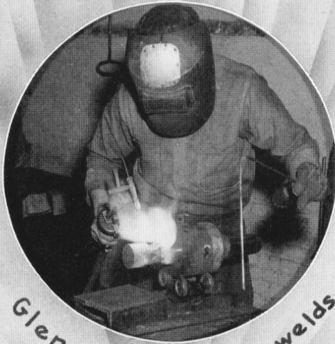
Ed Felburt uses torch to restore a broken cutter
